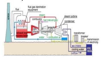
A combined cycle power first generates gas by burning fuel in the compressed air.
