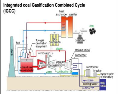
Integrated coal gasification combined cycle (IGCC) gasifies the fuel coal in the gasifier. Gasified fuel is burnt in the compressed air to generate gas. Pressure of the gas rotates the gas turbine to generate electricity. Furthermore the exhaust gas heat from gas turbine is utilized to boil water into steam to generate electricity.
