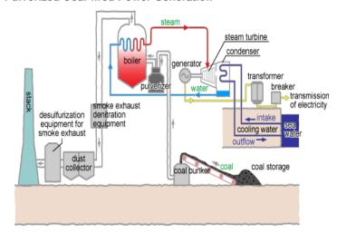
Pulverized coal-fired power generation is currently the major method of coal-fired power generation. Coal is pulverized to fine powder and is burned in the boiler. Heat in the boiler boils the water into steam. The steam pressure turns the steam turbine and the generator generates electricity.
